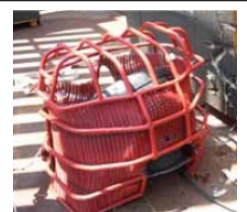
After >930 psi failure
